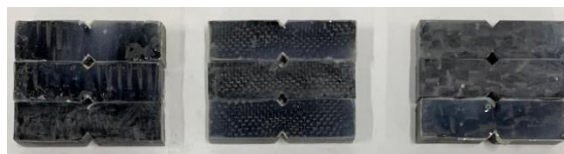
Gambar spesimen Uji Geser (dari kanan: spread tow , hexagonal , T300 )
