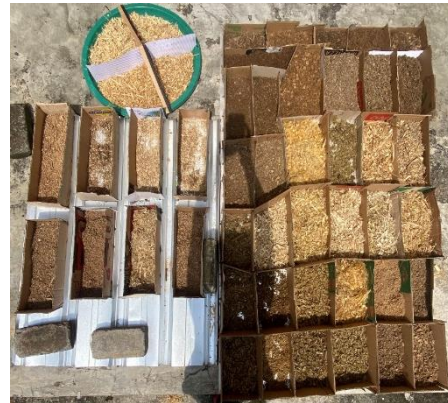
Gambar 4 proses penjemuran serat alam
