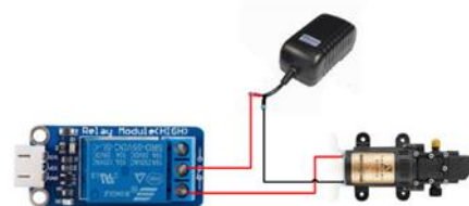
Gambar 22. Wiring TDS Water Quality
