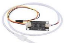
Gambar 5. Sensor TDS Water Quality
