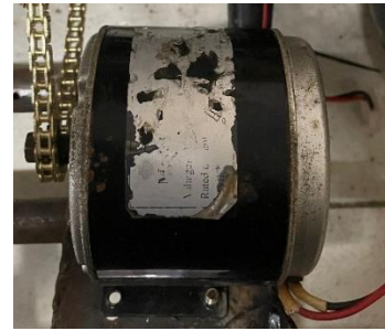
Gambar 18. Motor Listrik DC Shunt
