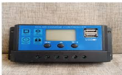
Gambar 9. solar charger ontroller
