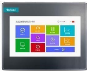
Gambar 2. Haiwell HMI SCADA
