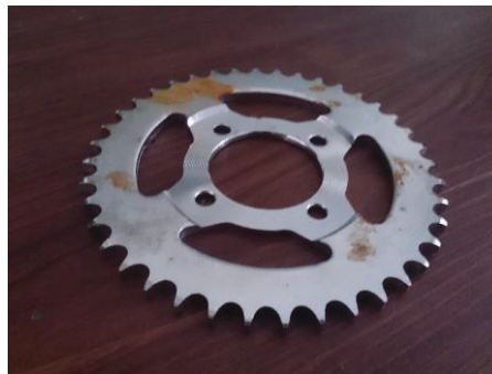
Gambar 6. Sprocket hasil powder metallurgy
