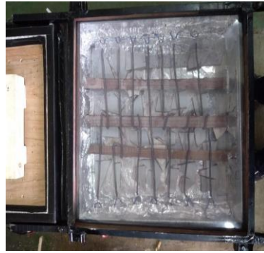
Gambar 7. Proses Pemanasan Lembaran Polystyrene diatas Heater
