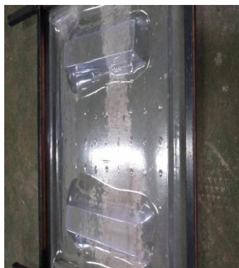
Gambar 11. Proses Pendinginan Lembaran Polystyrene
