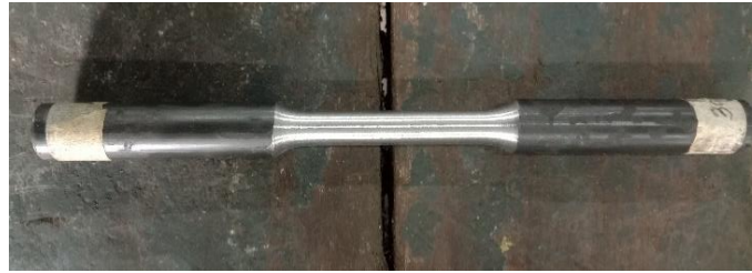
Gambar 3. Sampel Uji Tarik
