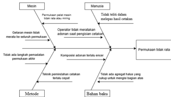
Gambar 4. Diagram Fishbone Cacat Ringan
